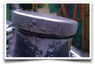
What is really noticeable is that it is the knurled surface that is succumbing most quickly to the attack - the polished top surface is staining, but not rotting away. Is there a metallurgical reason for this, anyone? Has the crushing effect of the knurling weakened the material or is it simply that the knurled surface collects and holds salty water? Now that I think on it, the alloy seat knobs went exactly the same way. They were replaced with stainless ones of a nice pattern from RGM.
